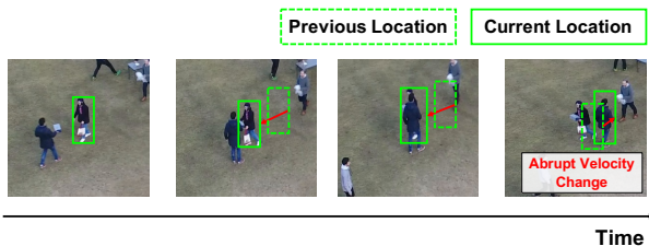
Fig. 6. Tracking failure due to occlusion leads to large acceleration.
